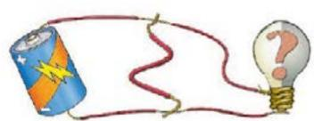
Students will need a circuit modified like the one shown in the illustration. (Strip a 1-inch section of insulation off the middle of each wire). Students will also need a 6-inch piece of thicker wire with 1 inch of insulation removed at each end.
